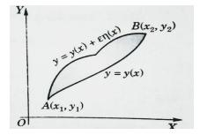
An integral such as (1), which assumes a definite value for functions of the type y = y(x) is called a functional. In diff. calculus, we deal with the problems of optimization of functions. The calculus of variations is however, concerned with optimizing functional.
