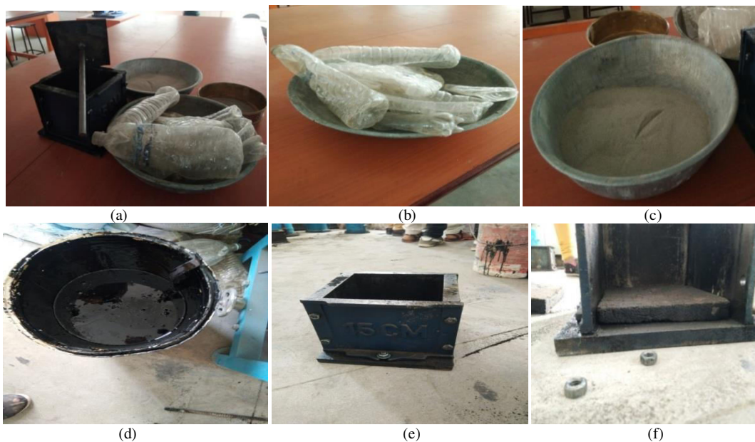
Fig. 2. a) Materials and mould, b) PET bottle, c) Fine quarry dust, d) Bitumen, e) Mould, f) Tile Specimen
