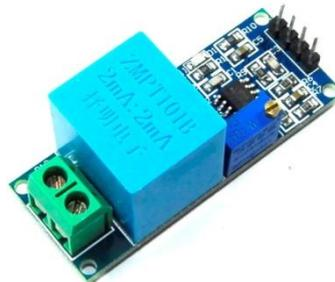
Fig.2. Voltage Sensor ZMPT101B
