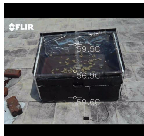
Figure 5.6 Spot temperature after Reflective sheet
