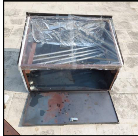
Figure 4.4 Solar dryer with reflective sheet
