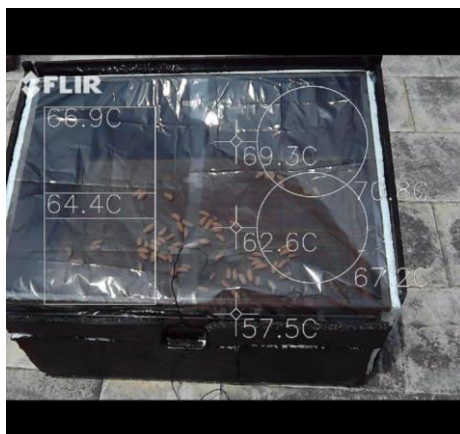
Figure 5.6 Spot temperature before Reflective sheet
