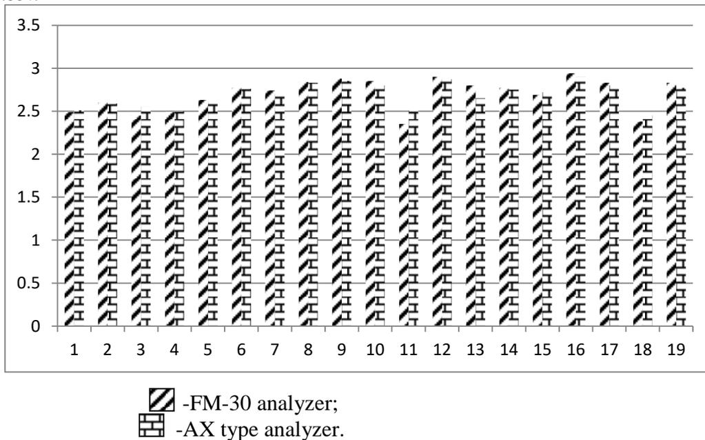
Figure 1. Results of determination of mass fraction of defects and contaminants in FM-30 and AX analyzers of type I State standard samples.
