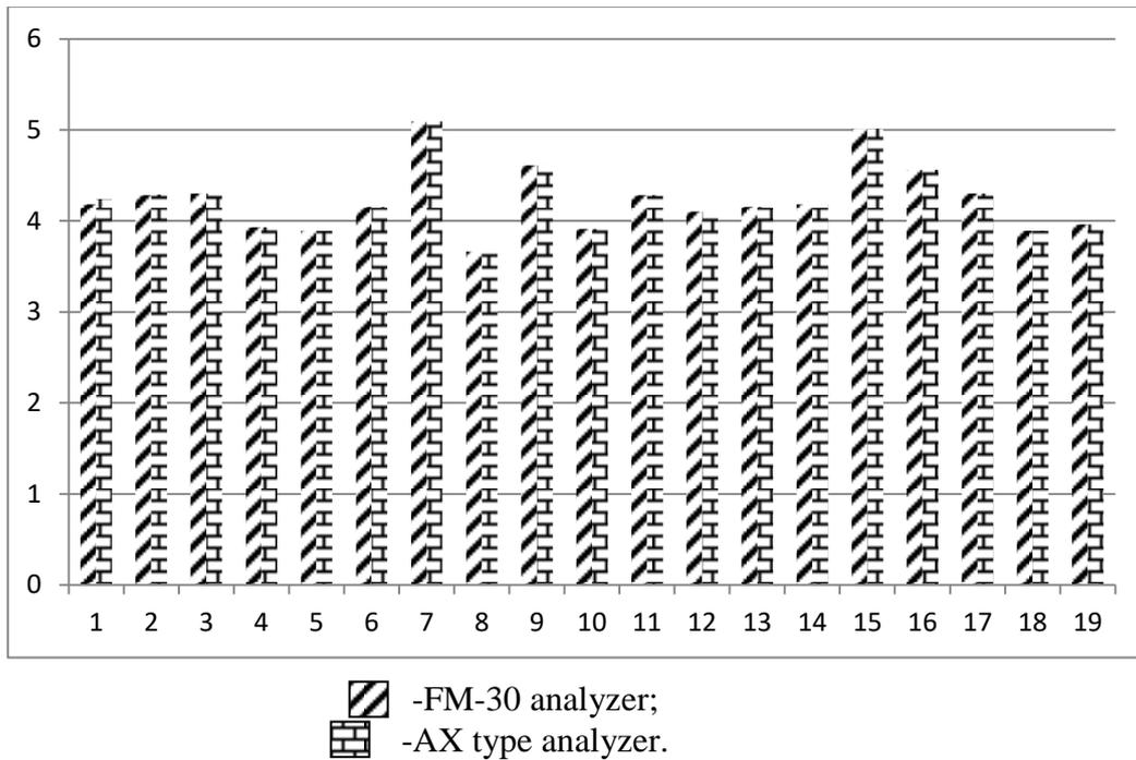
Figure 2. Results of determination of the mass fraction of defects and contaminants in the State Standard samples of type II in FM-30 and AX analyzers.
