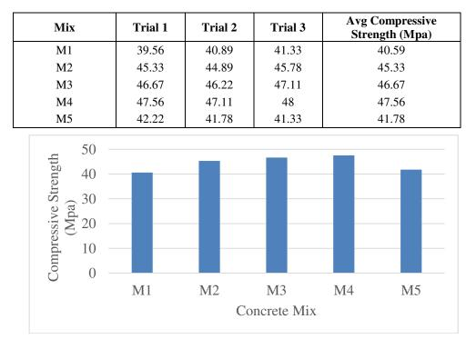
The compressive strength is evaluated by using the CTM. The above table and fig shows the strength of concrete at 28 days of curing period. The nominal mixed concrete has the compressive strength of 40.59MPa. As the percentage of fly ash increases upto 25% the value of compressive strength has increased to 47.56MPa. Above 25% the compressive strength decreases. The 30% replacement of fly ash has the compressive strength of 41.78MPa
