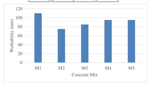
In the present investigation the workability of concrete is measured by slump test. The workability of concrete without any admixtures shows the slump value 110mm. By using 10% of fly ash and 1% of polypropylene fibre the workability reduces to 75mm, but as the percentage of fly ash increases for the other trials the slump value gradually increases. So the replacement of 25% and 30% the slump value is 95mm.
