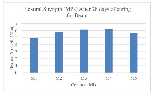
The Flexural strength is evaluated by using the CTM. The above table and fig shows the strength of concrete at 28 days of curing period. The nominal mixed concrete has the Flexural strength of 4.97MPa. As the percentage of fly ash increases upto 25% the value of Flexural strength has increased to 6.23MPa. Above 25% the Flexural strength decreases. The 30% replacement of fly ash has the Flexural strength of 5.65MPa
