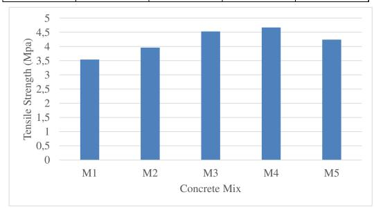
The Tensile strength is evaluated by using the CTM. The above table and fig shows the strength of concrete at 28 days of curing period. The nominal mixed concrete has the Tensile strength of 3.54MPa. As the percentage of fly ash increases upto 25% the value of Tensile strength has increased to 5.09MPa. Above 25% the Tensile strength decreases. The 30% replacement of fly ash has the Tensile strength of 4.24MPa.
