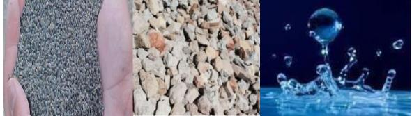
Coarse aggregates are the stone pieces which are obtained by crushing the stones in a crusher or from the river banks. Coarse aggregates are retained by 4.75 mm of IS sieve.
