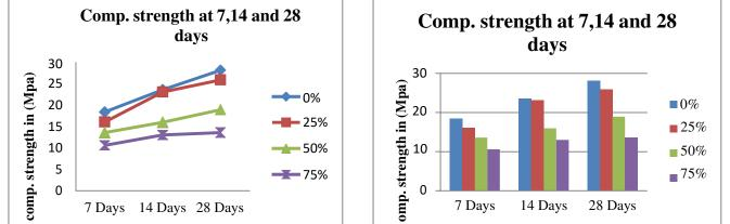
The Compressive Strength of RAC where Aggregate is replaced by Recycled Aggregate with proportion 0%, 25%, 50% and 75% on 28 days curing is 28.17 Mpa, 25.9 Mpa, 18.93 Mpa 13.6 Mpa respectively.
