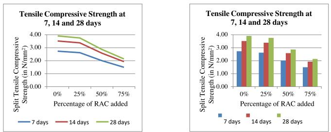
The Split Tensile Strength of RAC where aggregate is replaced by Recycled Aggregate in proportion 0%, 25%, 50% and 75% on 28 days curing is 3.93 Mpa, 3.77 Mpa, 2.89 Mpa and 2.17 Mpa respectively.
