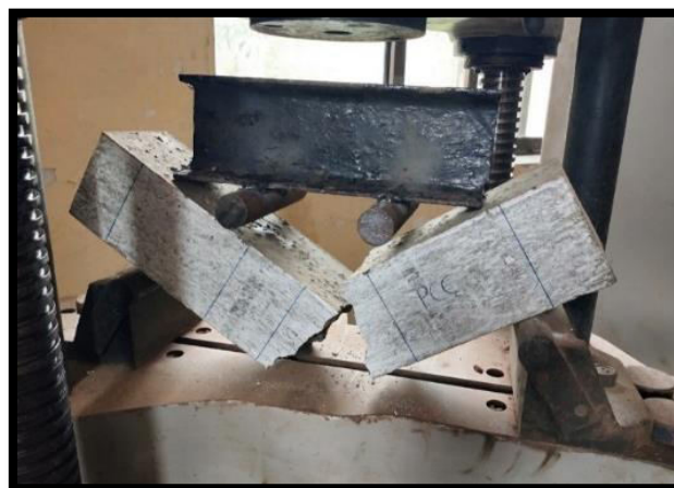
Fig3: Failure pattern of plain cement concrete
