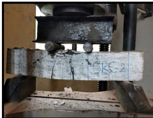
Fig5:Failure pattern of steel reinforced concrete (Doubly reinforced beam)
