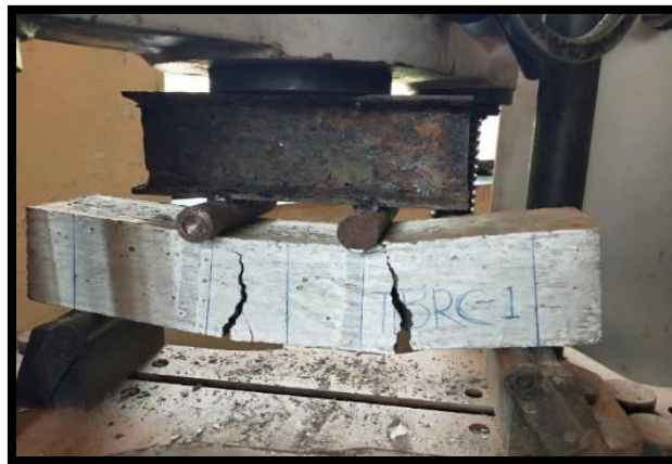
Fig8:Failure pattern of treated bamboo reinforced concrete coated with tar (Singly reinforced beam)
