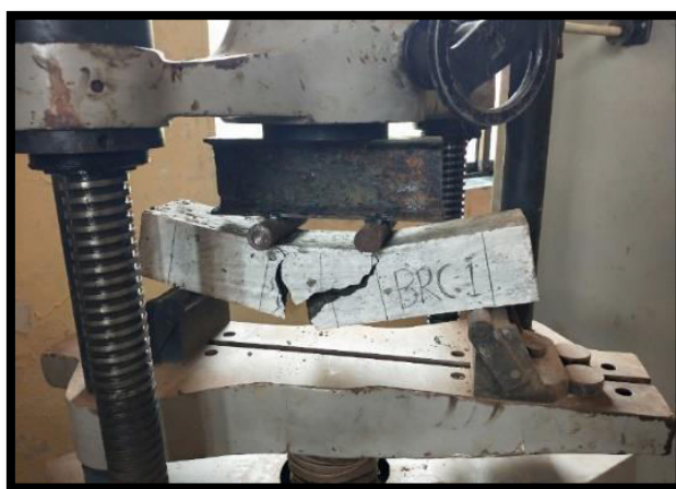
Fig6:Failure pattern of bamboo reinforced concrete (Singly reinforced beam)
