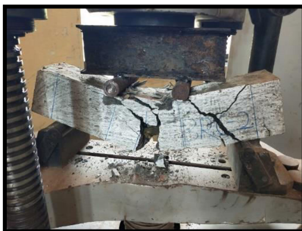
Fig7:Failure pattern of specimens consisting bamboo reinforcement (Doubly reinforced beam)
