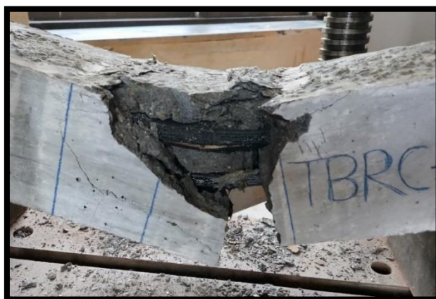
Fig10: Failure of treated bamboo reinforced concrete coated with tar
