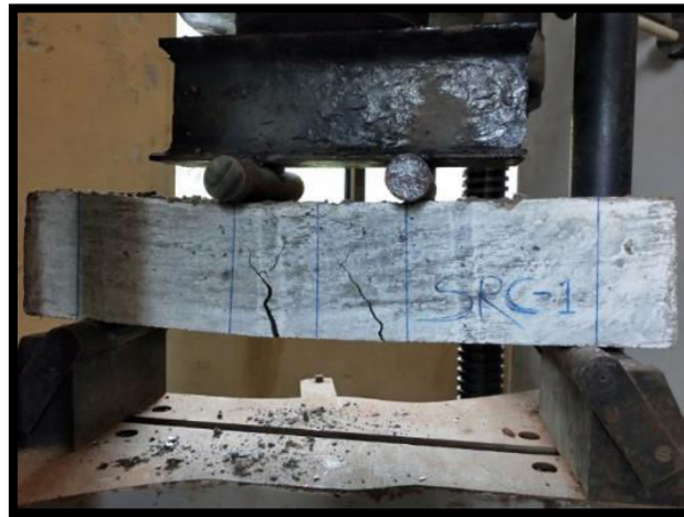
Fig4:Failure pattern of steel reinforced concrete (Singly reinforced beam)
