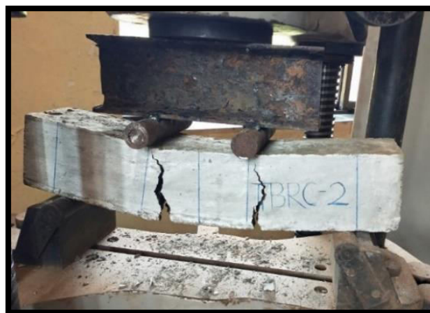
Fig9:Failure pattern of treated bamboo reinforced concrete coated with tar (Doubly reinforced beam)
