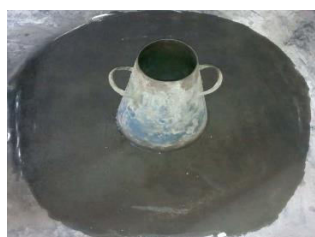
(a) Slump flow test conducted for self-compacting concrete
