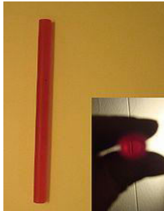
A ruby laser rod. Inset: The view through the rod is crystal clear
