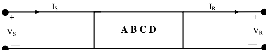
Figure 3.3: Two-port representation of a transmission line.
