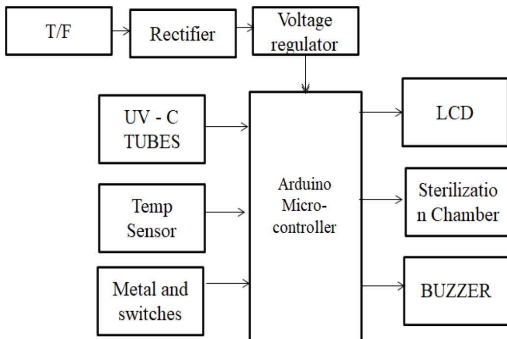
**Figure .1. Basic Block Diagram**
