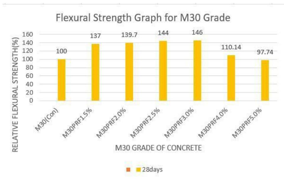
Figure No.6. Graph of Flexural Strength of M30 Grade With Different Dosage of Polyester Recron Fibre
