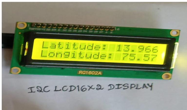
Figure 6: Display message on LCD
