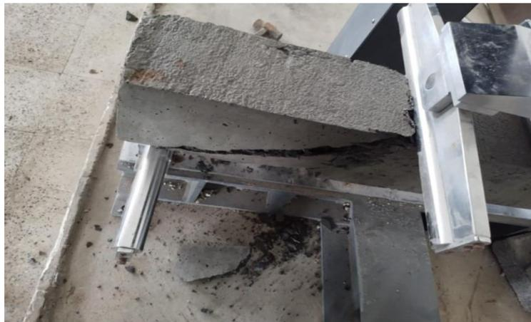
Figure 3a Failure pattern of Reinforced Concrete Beam
