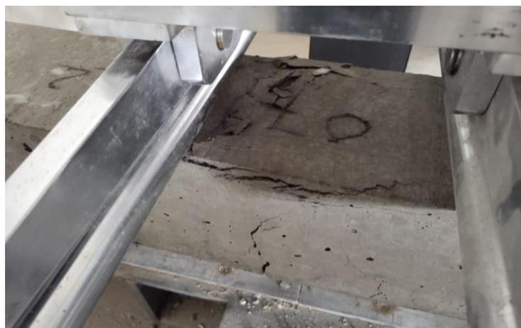
Figure 3b Failure pattern of Reinforced Concrete Composite Beam-1
