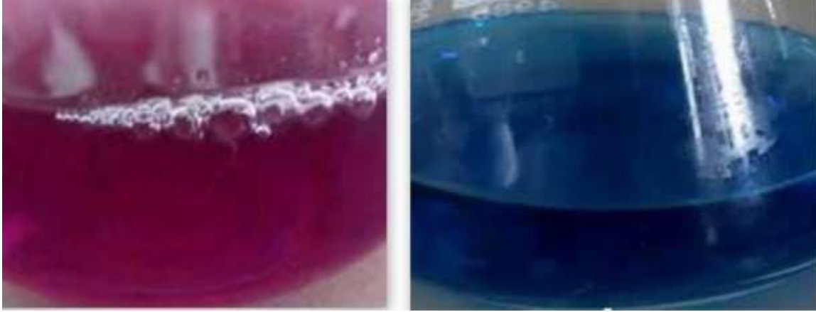
Figure 3: Determination of end point of Ca 2+ (colour changes from purple to blue).
