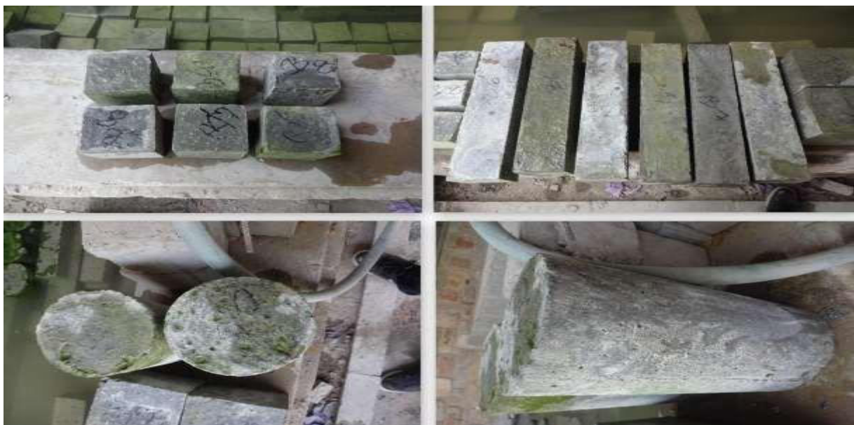
Figure 1: Concrete specimens of cubes, beams and cylinder.
