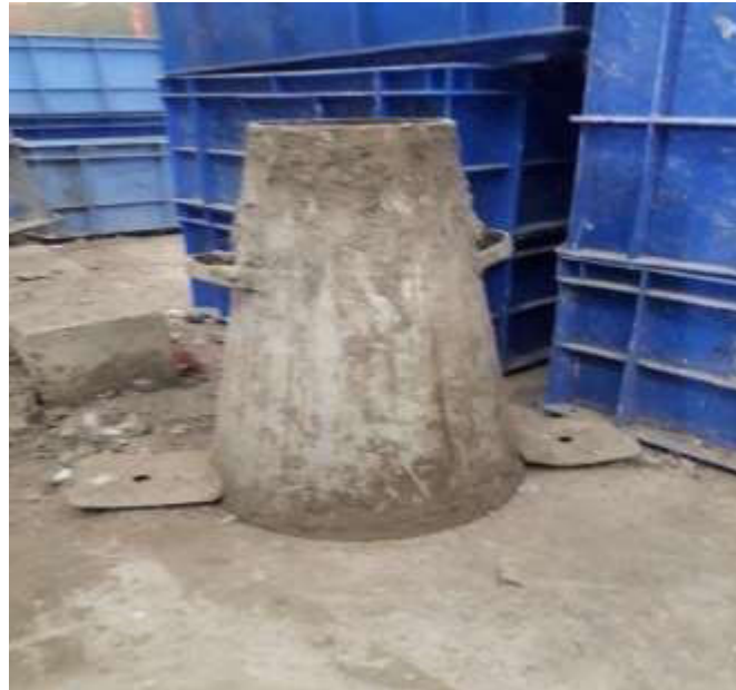
Figure 6: Slump cone test for workability
