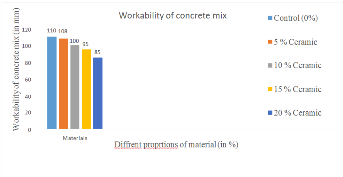
Figure 5: Workability of concrete mix with different proportions of ceramic waste
