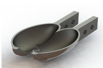
Figure 3 Pelton Turbine Bucket In Isometric View
