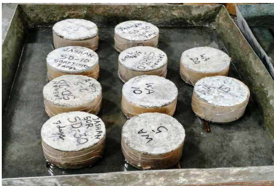
Figure 4 sorptivity test of mortar samples
