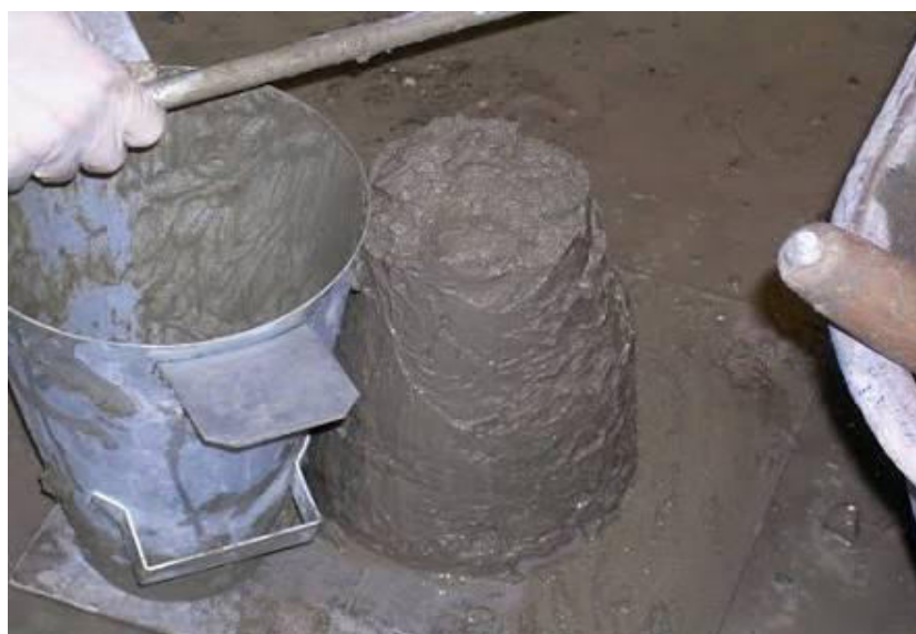
Figure 1: slump test of mortar
