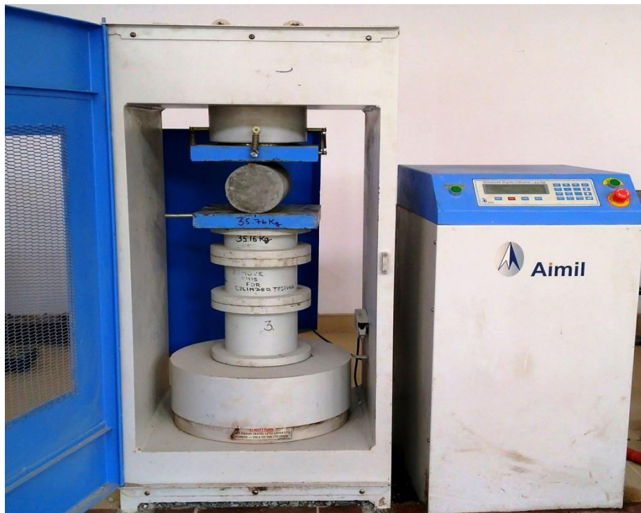
Figure 3: splitting tensile strength test of mortar
