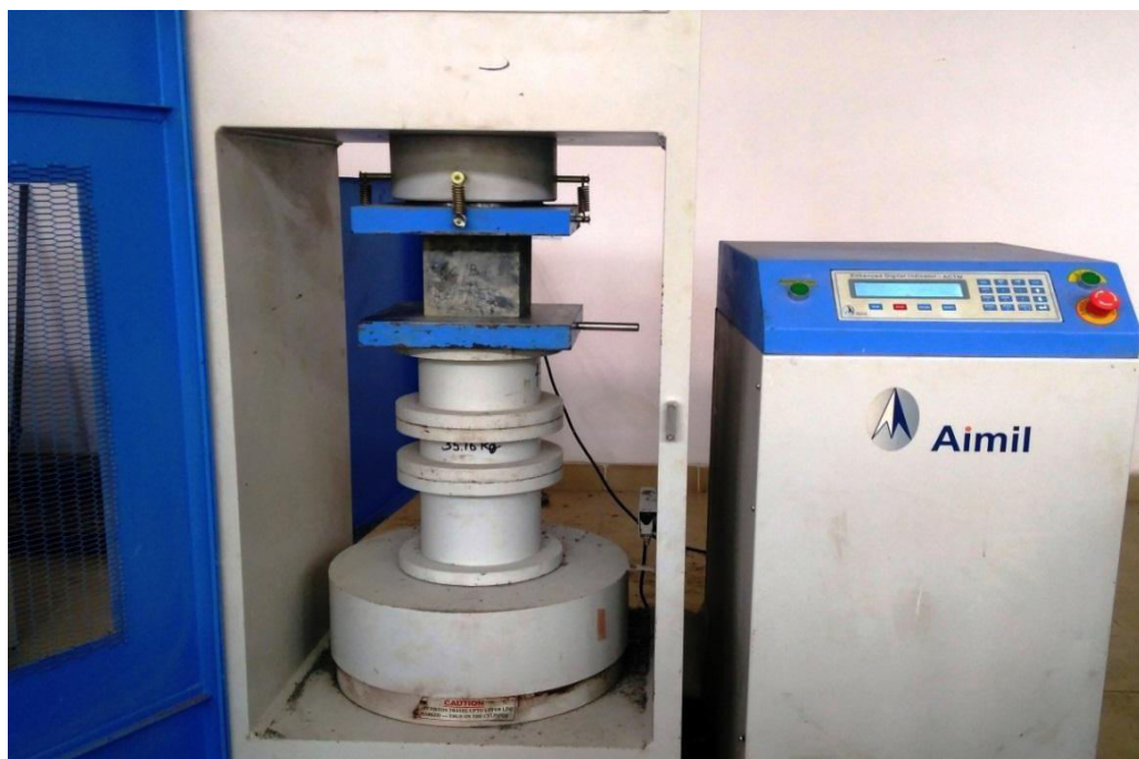
Figure 2: compactionstrength test on compression testing machine
