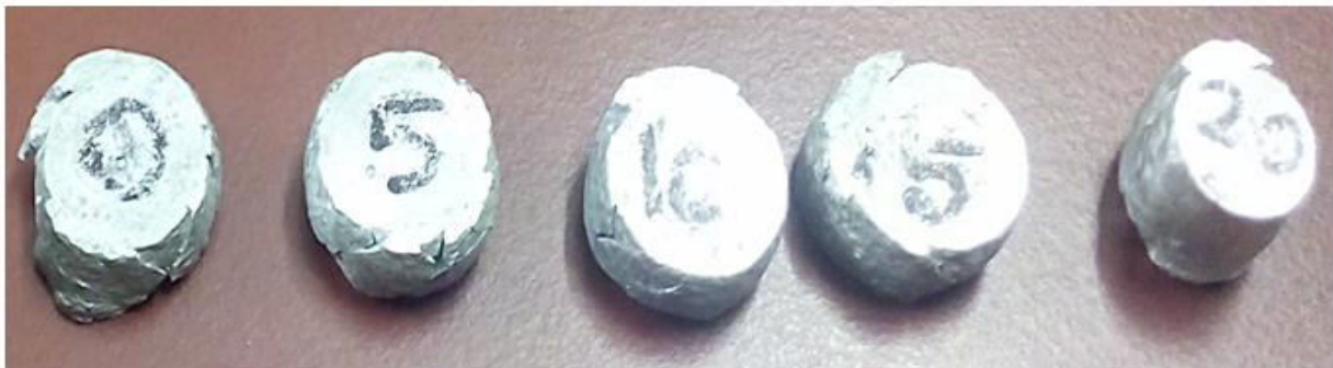
Fig. 3. Compression test specimens after test
