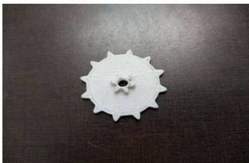
Fig 5.3.2: Printed Coded Gear.
