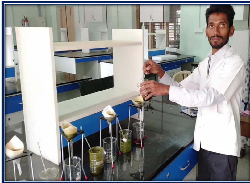
Figure.2.5. 10 ml of Bullet Woodleaf extract was added Drop wise to 5 ml of 1 mm silver nitrate solution.
