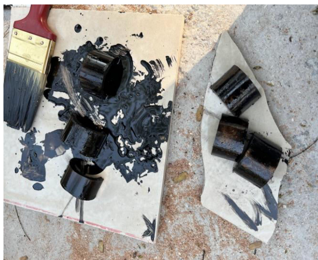
Figure 3: Test Specimens for Water Absorption Test - Bamboo surface treated with Black Japan paint
