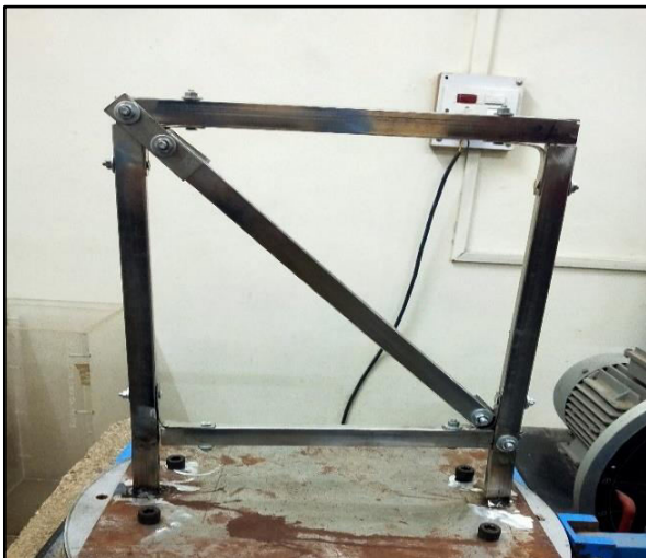
Figure 2 With & Without Infill Wall Test on Shake Table
