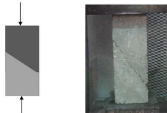
Figure 5. Slant shear test
