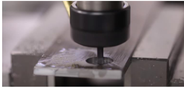
Fig.6 Titanium cutting using PCNC 440 CNC mill
