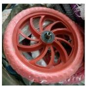
In Mechanical Electric two tyres is used in both the sides. Scooter wheels are used in Electric reason behind that cost is less, easily available and friction property is also less. Also higher amount of weight gaining capacity and movements is also very smooth.
