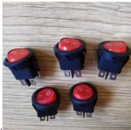
It is used to guide the direction of rotation of motor shaft. By operating the switch the direction of vehicle can be controlled. Connecting wires are used to connect switch with motor.
