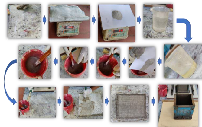
Figure 3.1: GFRP with Prosopis juliflora lamination
