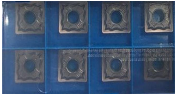
Fig 3: Titanium coated carbide inserts
