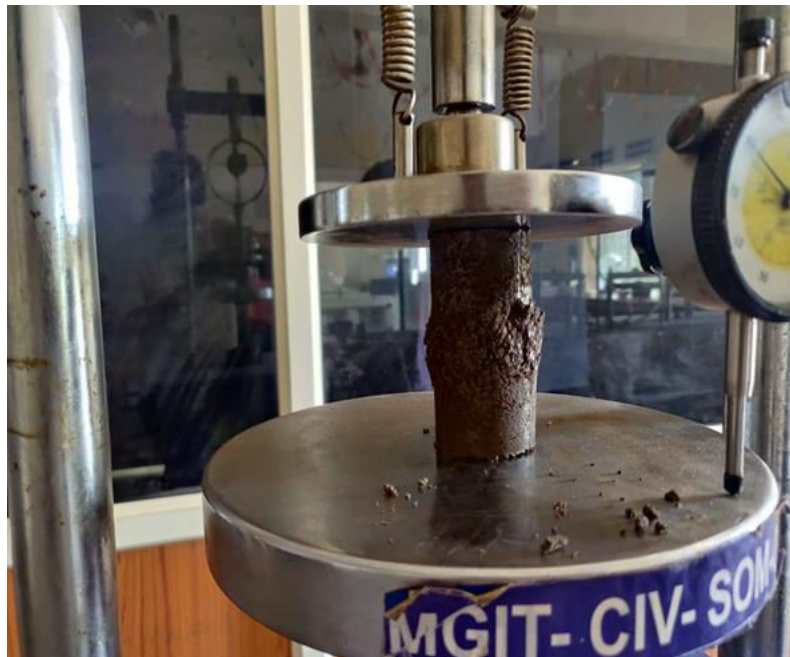
Fig.2 unconfined compression test
