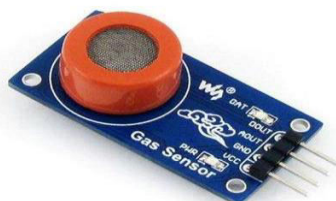
Fig.5. Pin configuration Alcohol Sensor
