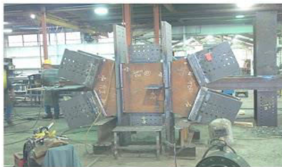
Figure no.6 : A Diagrid node after fabrication
