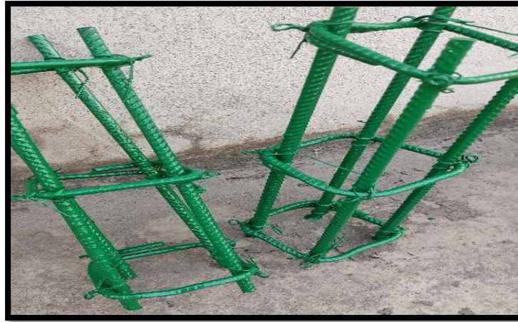
Fig 1-Making of coating procedure on TMT bars
