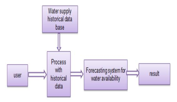
In above block diagram we are going to give user input and water supply historical data base for processing block which will process or forecast using some machine learning algorithm and this processed data is available for water forecasting then will get actual result.
