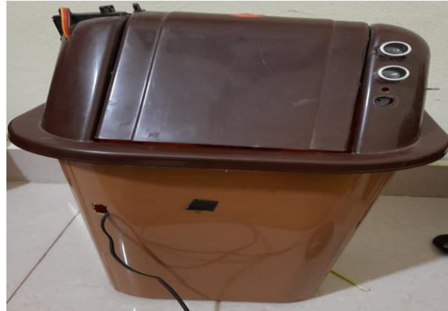
Fig6Automatically Operating dustbin ready
