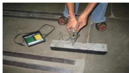
Fig. Rebound Hammer Test
