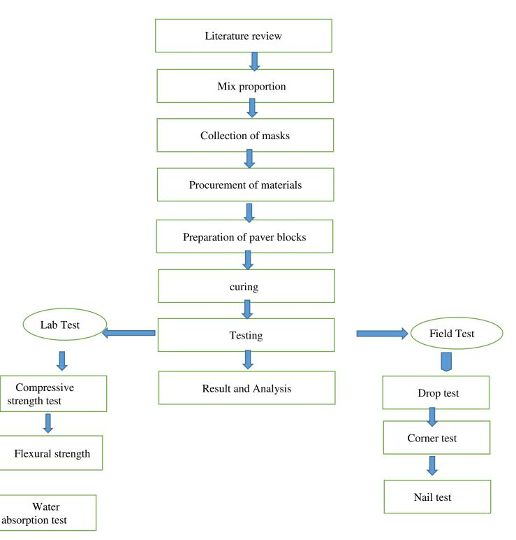
The various steps used in preparation of pavement blocks are as follows:
