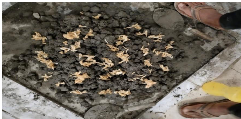
Fig No. 1 Cigarette butts Added in Concrete
