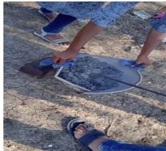
MIXING OF PET BOTTLE PAVEMENT BLOCK
