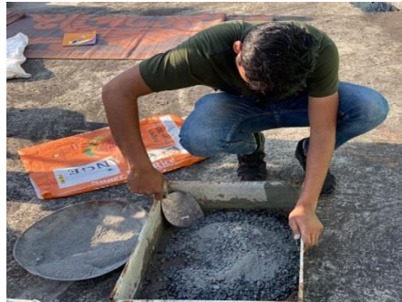
MIXING OF QUARRY DUST PAVEMENT BLOCK
