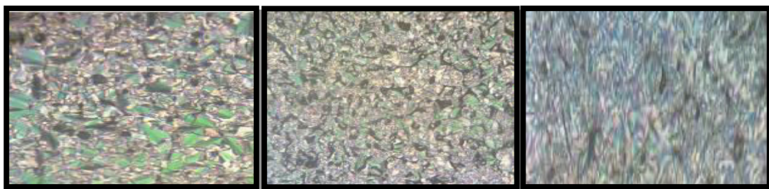
Figure 3. Optical textures of ligand under a polarizing optical microscope
