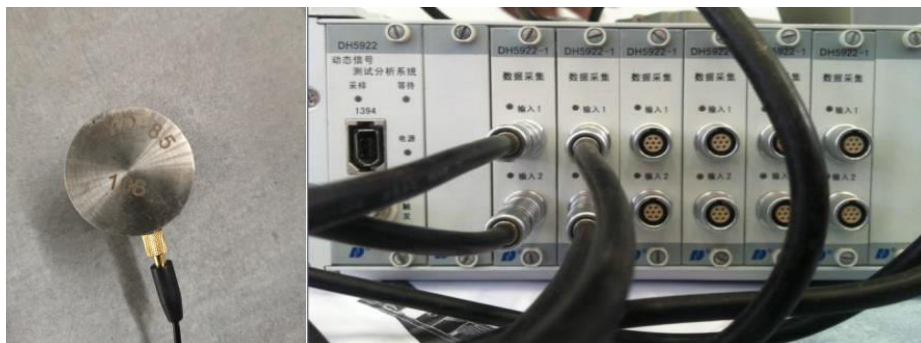
Fig.4. Acceleration sensor and data acquisition system
