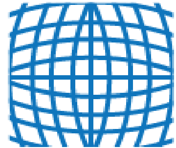
Barrel distortion Negative radial displacement
