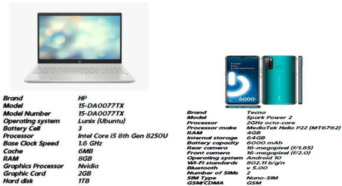
Figure 5. Specifications of the Laptop Computer (a), Specifications of the Smart Phone (b)
