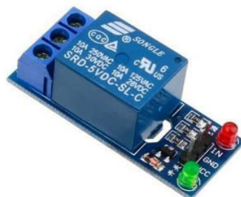
Fig. 7. Relay Module (SRD-5VDC-SL-C)
