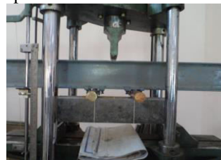
Fig. 6.3.2: Flexural test on concrete
