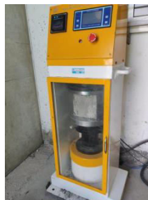
Fig. 6.1: Compression test on concrete
