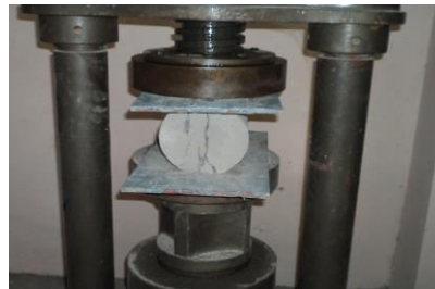
Fig. 5.3.2: Split tensile test on concrete
