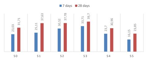
• Compressive strength of control concrete and concrete made by replacing M-sand with copper slag at various percentages
