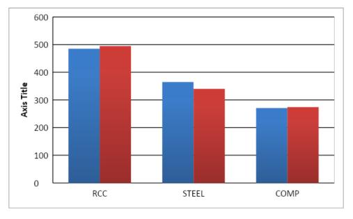
From above comparison its found that the shear gradually decreases from RCC to steel and but finally at composite shows better performance in the reduction of the Shear when compared with that of all other model.
