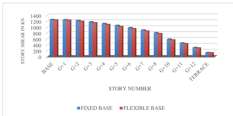
Fig 8. Story shear for G+12 building zone v, soft soil
