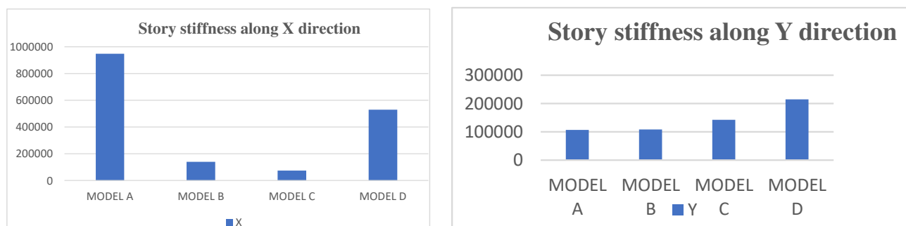
Fig-4.4 Story stiffness along X and Y direction of all 4 models
