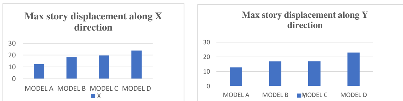
Fig-4.1 Max story displacement along X and Y direction of all 4 models
