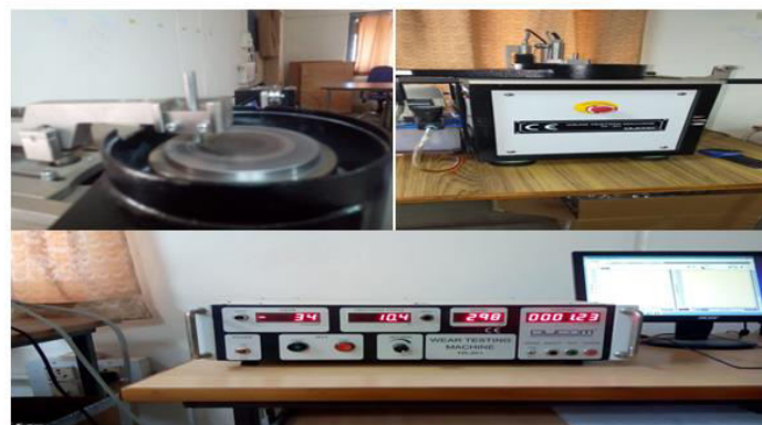
Fig 3.2 (a): pin-on-disc wear testing apparatus
